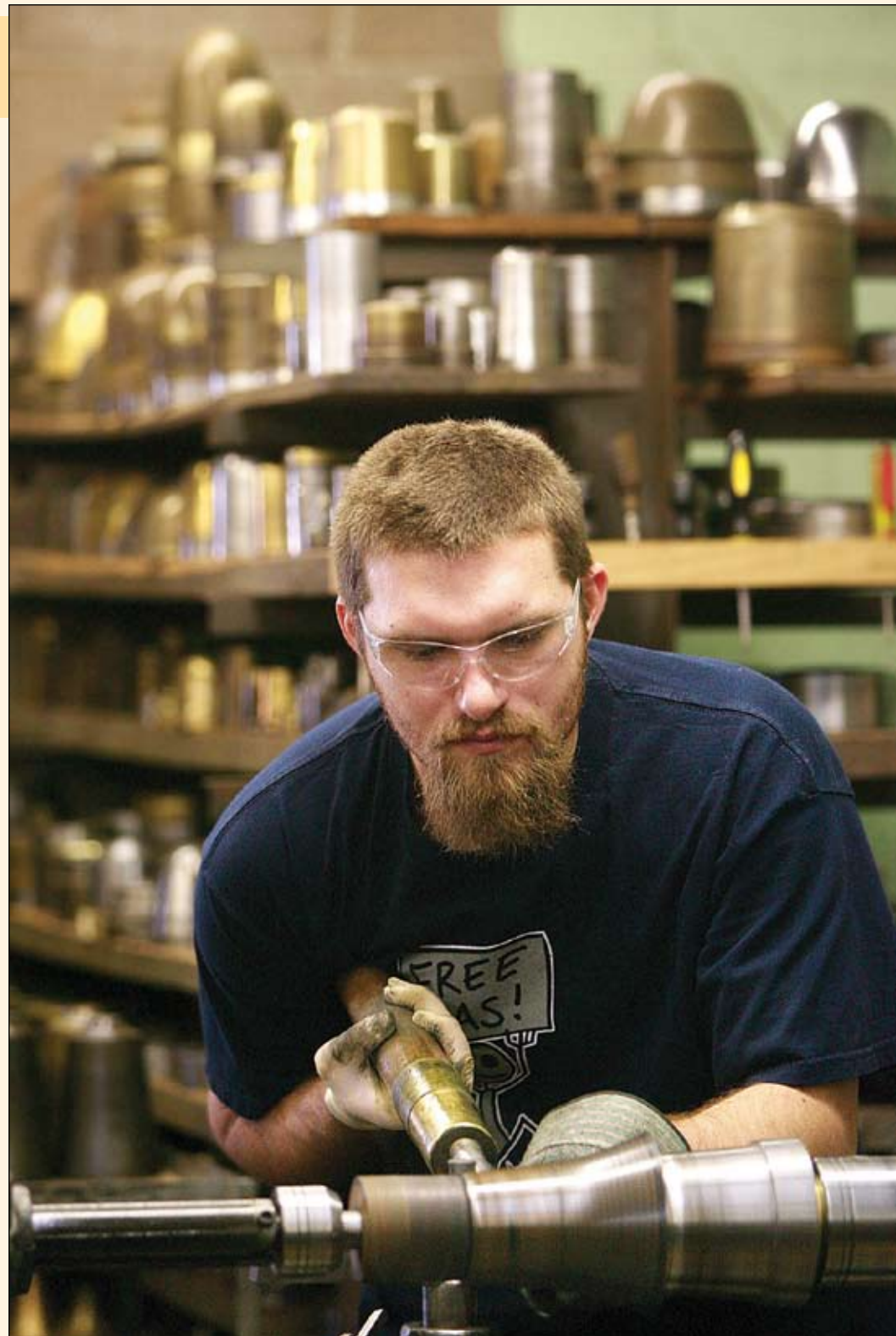
Greg St. Claire forms a holy water bucket on a spinning lathe.
